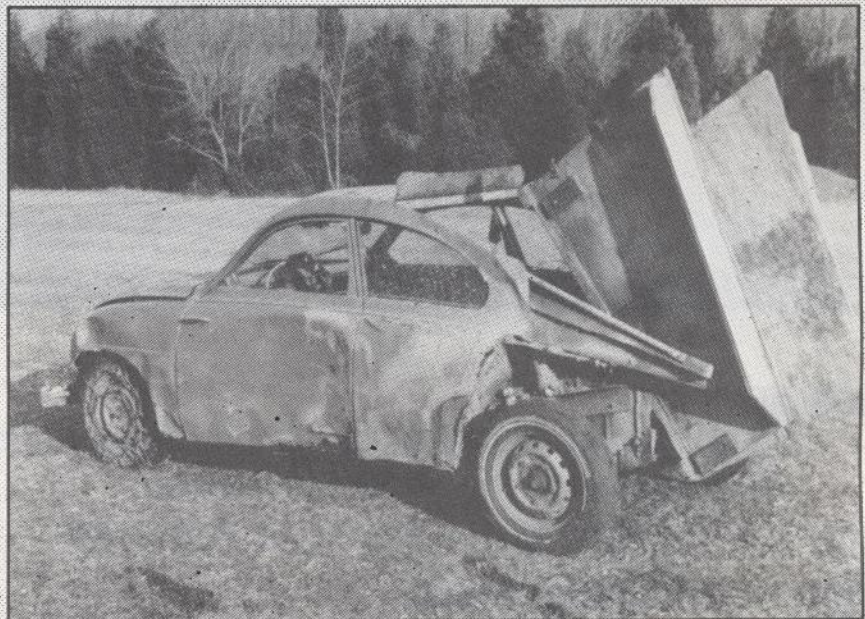
Late 1950's SAAB 93B "dump truck". The front bumper is a 4-inch log, it has chains for added traction, and a custom-designed roof-airfoil to divert unwanted breezes.
