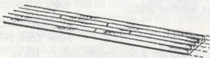
Figure 1. Minor cracks in the ribs do not affect the performance of the belt.
