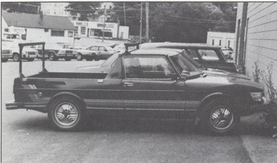
SAAB Pickup, built by Mike Billing at Clyde Billing SAAB in Augusta, Maine. The front is from a '78 99, the rear an '86 900. 6" was added to the wheelbase. The bed frame is made of 2"x4" steel. This is the second SAAB truck constructed at Billing SAAB (the first one is for sale). photo by Tim Winker.
