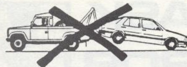
Do not use sling-type equipment to tow 1989 9000 models.
