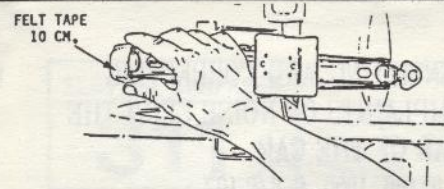
Figure 5. Installing felt tape on the jack.
