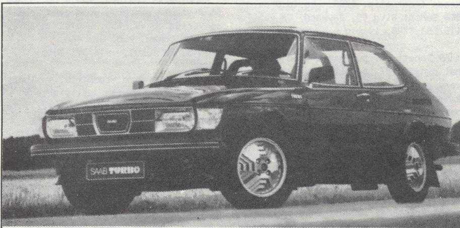
Introduced in 1978, the SAAB 99 Turbo is credited with starting the trend of turbocharging smaller sedans.
