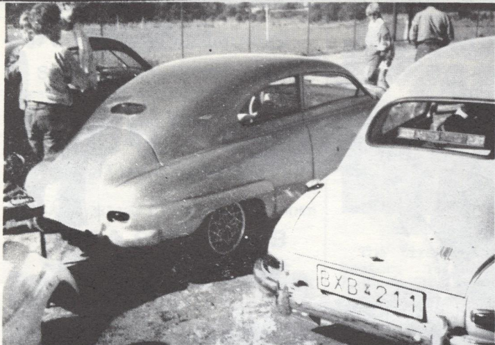
Above left & right: "Blue Flame", a chopped and lowered '59 93B. Note the integral bumpers, "frenched" signal lights, and one-piece hood. Below left & right: Stretched 95 with a hand-made hood, powered by a Ford V6. Also, a "dressed up" Cabriolet with gold plated trim.
