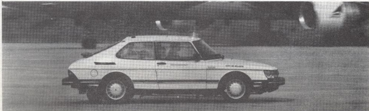
Atlanta Airport's Saab Friction Tester measures friction on runway surfaces to help pilots land under critical weather conditions.
