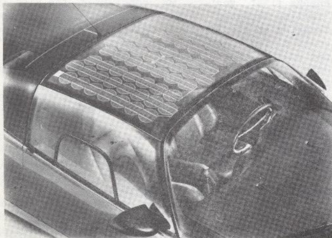
Solar cells in the roof provide power to interior cooling fans.
