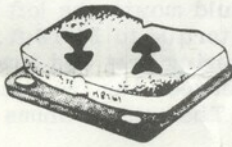
Semi-metallic brake lining up to and including 1982 model. ONLY for outside of brake disc.
