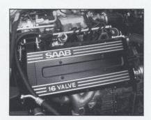
placement increase of 100 cc would hardly seem worth the effort, but the real-world result is a noticeable improvement in bottom-end and midrange passing performance far in excess of the modest increases in horsepower (up to 140 bhp from 128) and torque (a 5-lb.-ft. jump to 133).
